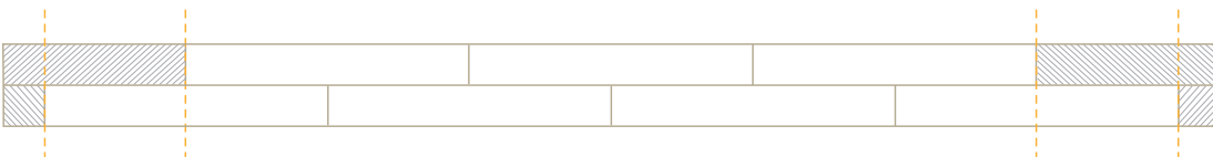
Figure 11: Gluing down initial rows with reference lines and fitted pieces.
